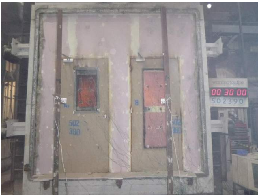
Figure 37 Unexposed face of the specimen after a test duration of 30 minutes
