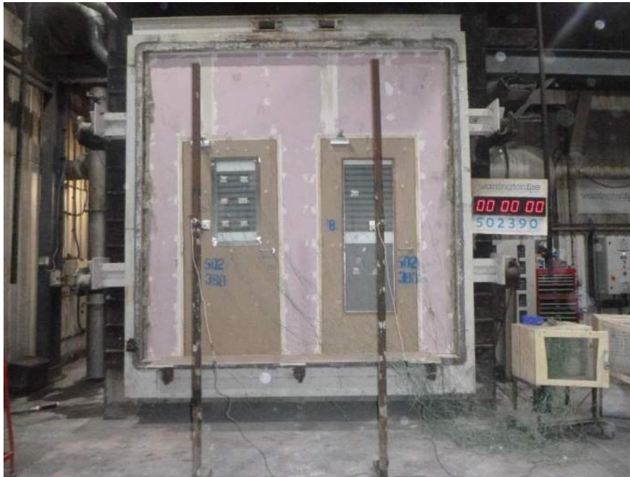
Figure 34 Unexposed face of the specimen before the start of the test
