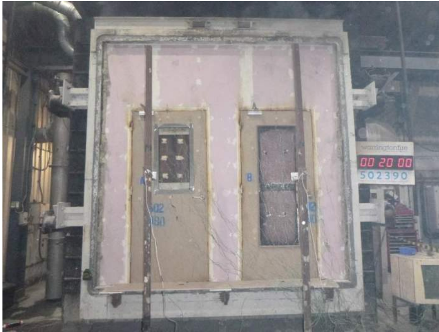
Figure 36 Unexposed face of the specimen after a test duration of 20 minutes
