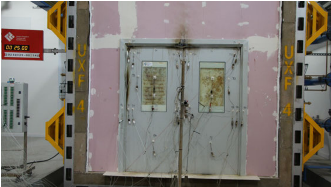
Figure 19 - The unexposed surface of the test construction after a test duration of 25 minutes
