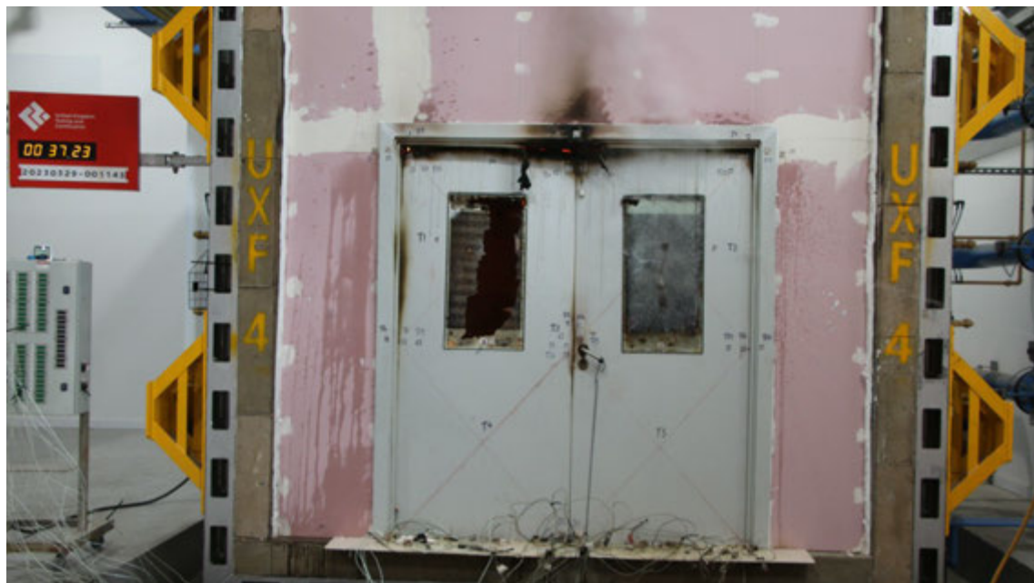
Figure 22 - The unexposed surface of the test construction after a test duration of 37 minutes
