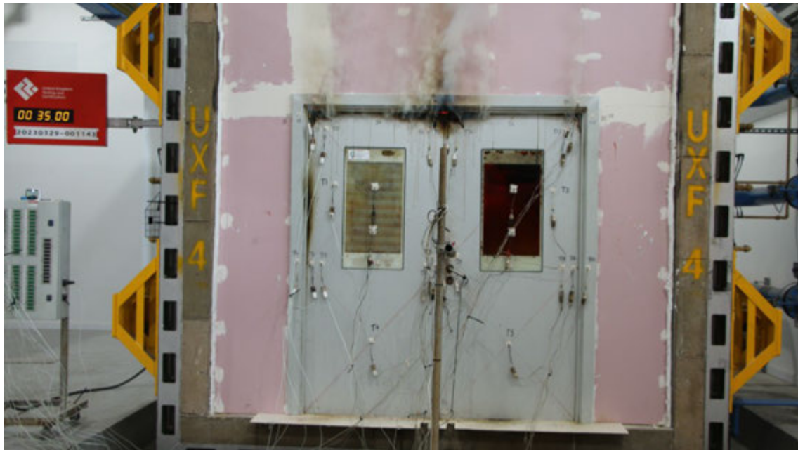
Figure 21 - The unexposed surface of the test construction after a test duration of 35 minutes
