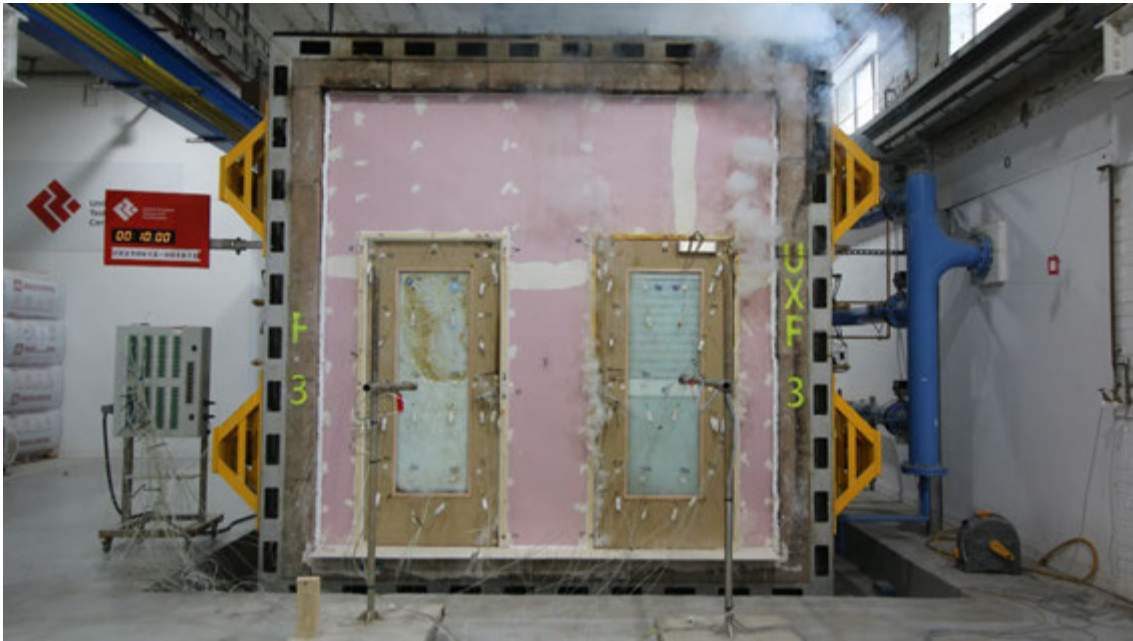
Figure 17 - The unexposed surface of the test construction after a test duration of 10 minutes
