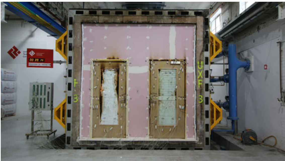
Figure 22 - The unexposed surface of the test construction after a test duration of 39 minutes
