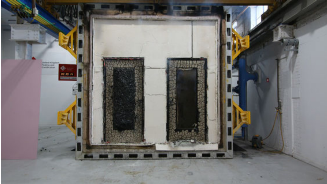
Figure 23 - The exposed surface of the test construction after the test was discontinued
