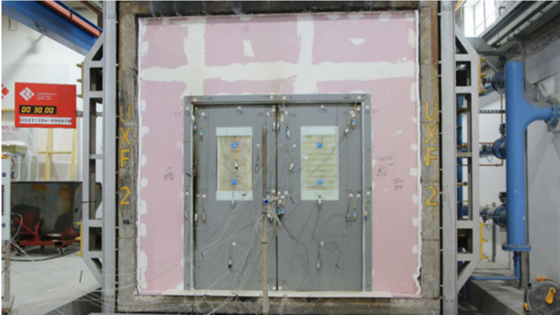
Figure 19 - The unexposed surface of the test construction after a test duration of 30 minutes
