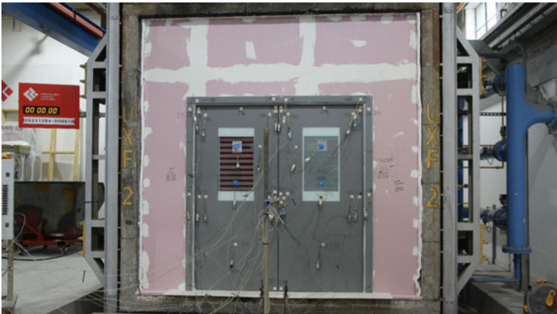
Figure 16 - The unexposed surface of the test construction prior to the commencement of the test
