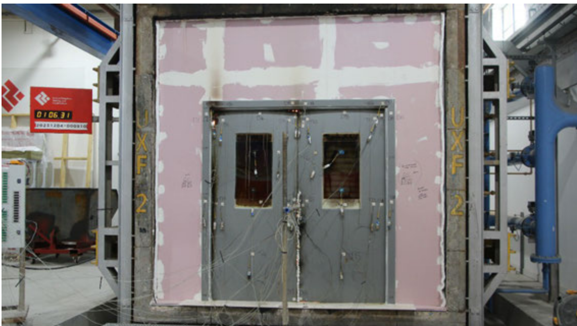
Figure 24 - The unexposed surface of the test construction after a test duration of 66 minutes
