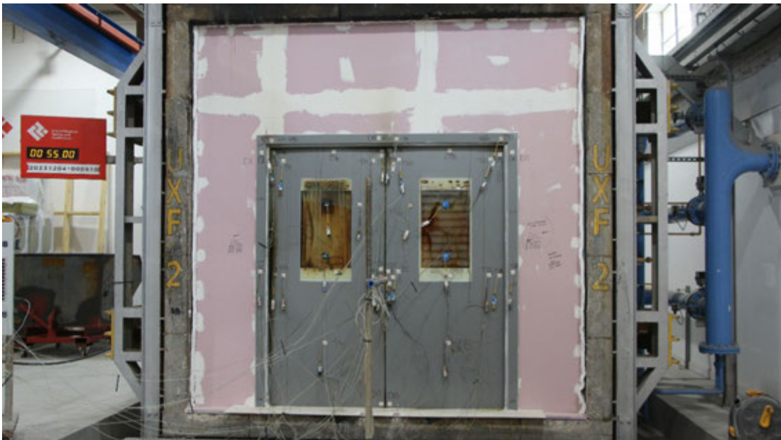
Figure 22 - The unexposed surface of the test construction after a test duration of 55 minutes
