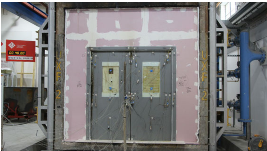
Figure 20 - The unexposed surface of the test construction after a test duration of 40 minutes
